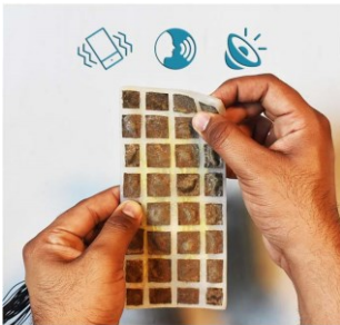
(b) Deformation gesture-based interaction on a smartphone-sized flexible device
